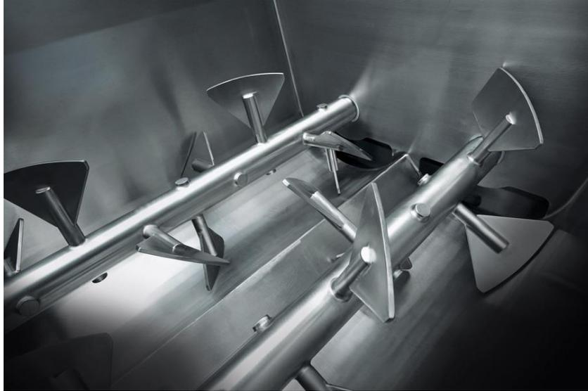
A gentle, intensive mixing process is achieved with two separately controllable mixing paddles.
